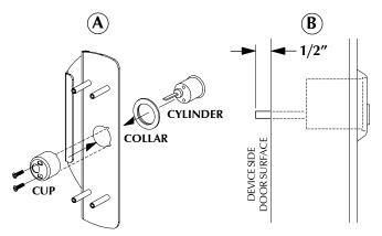
INSTALL EXIT DEVICE AND TRIM (INSTALL TAILPIECE GUIDE IF USING A CYLINDER).
