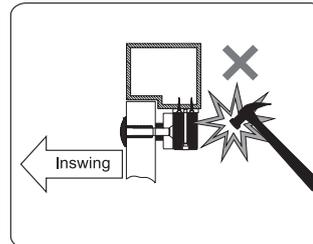
Be aware that it is better to install the electromagnet lock inside the house and hide the cable inside the door frame in order to guard against unlawful entry. With LZ for inswing doors.
