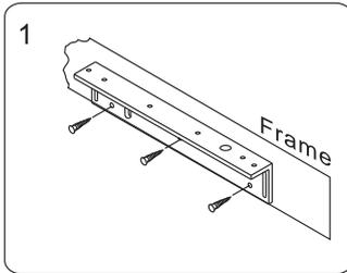
1 Find a mounting position on the door frame for the L bracket. Make sure that the door can still be closed.
