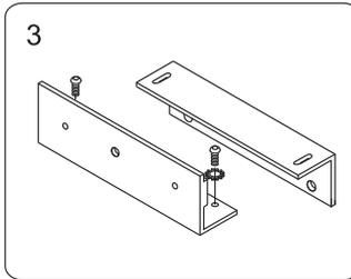
3 Assemble the Z bracket and make sure that the Z bracket is adjustable.
