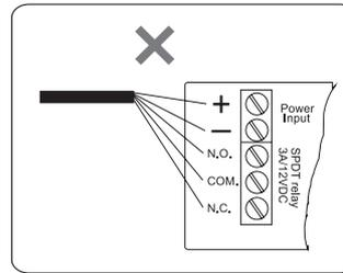
Do not apply power wires and signal wires in the same cable or conduit.
