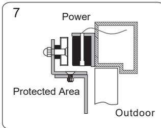
7 After the magnet attracts the armature plate, adjust the Z bracket to fit the door.
