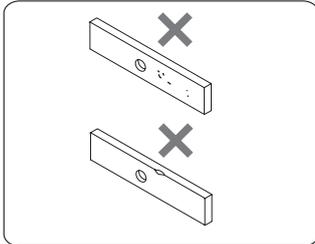
Make sure the contact area of the electromagnetic lock and the armature plate are clean or the bond sensor output function will not work.
