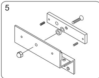
5 Attach the armature plate and washers to the Z bracket assembly.
