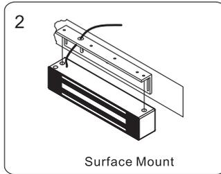
2 Use the fixing bolts to tighten the magnet on L bracket.
