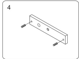
4 Insert the guide pins into the armature plate.
