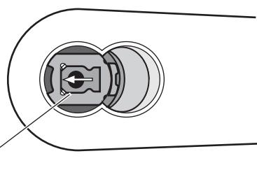
Using a flat-blade screwdriver, remove the lever by pressing on the lever keeper.
