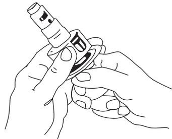
5. Depress slide, unhook old, remove both inside plunger and spindle.
