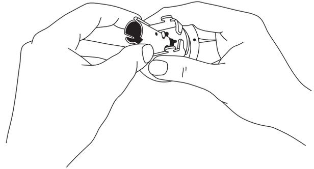
10. Reposition hub plate slide and springs in frame.
