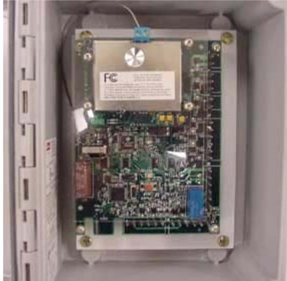
**Figure 6-16 – Removing the WRI-OTD-12VDC PCB**
