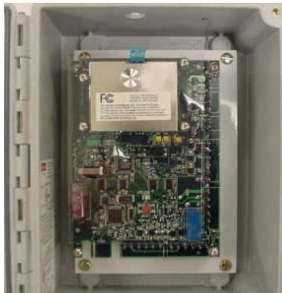
**Figure 6-19 – Replacing the WRI-OTD-12VDC’s PCB**
