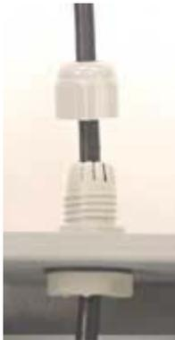
**Figure 6-15 – Securing the PIM's Antenna NEMA Gland**
