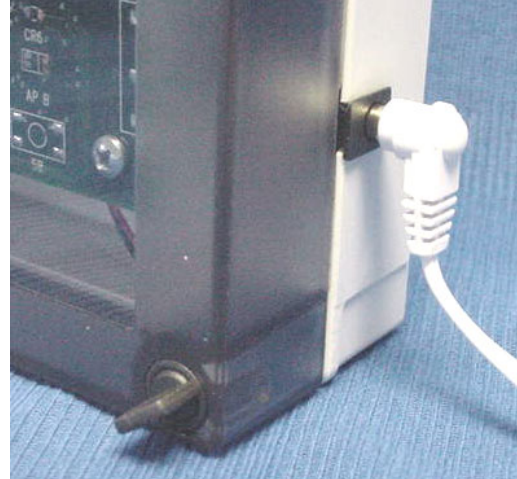
Figure 2-3 – Original PIMT PCB Power Connections
