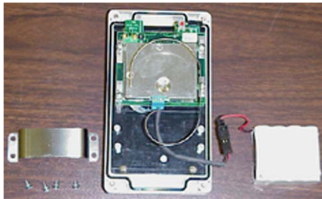
Figure 2-3 - Installing New Battery Pack
