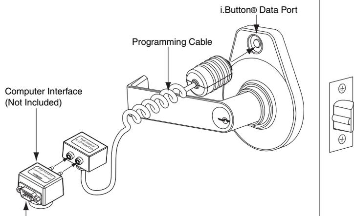
For 9-Pin Cable connection to computer
