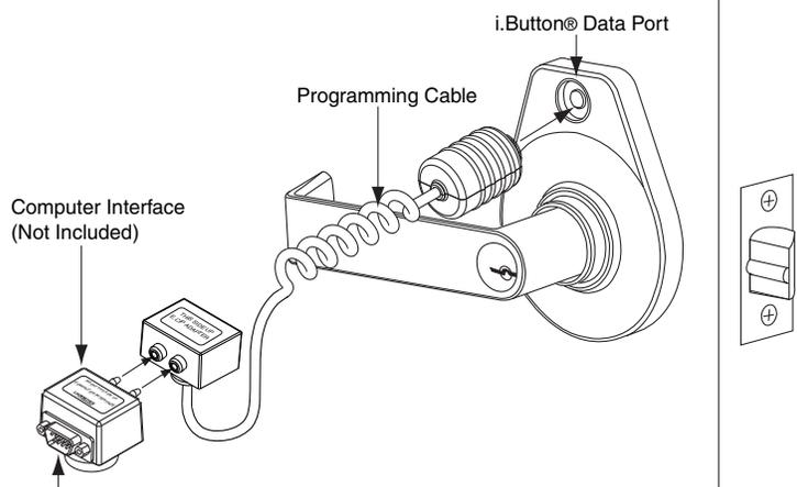
For 9-Pin Cable connection to computer
