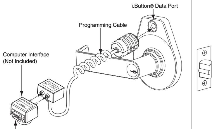
For 9-Pin Cable connection to computer
