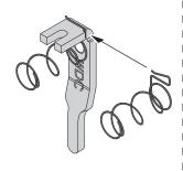
With device center case hanging over edge of table, insert lift finger with spring compressed thru upper block of center case.
