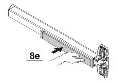
Loosen the top adjustment locking screw.
