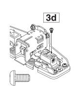
Press lift finger screw upward to preload spring (3e).
