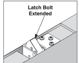
With pushbar depressed, latch bolt should be flush with top edge
