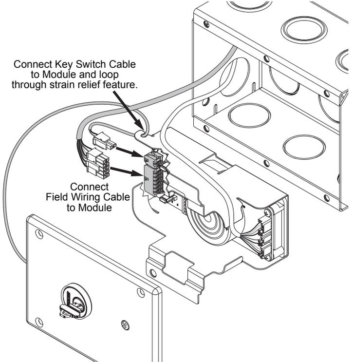
7q Insert mounting bracket with module into control box and screw into place. Screw faceplate into place.
