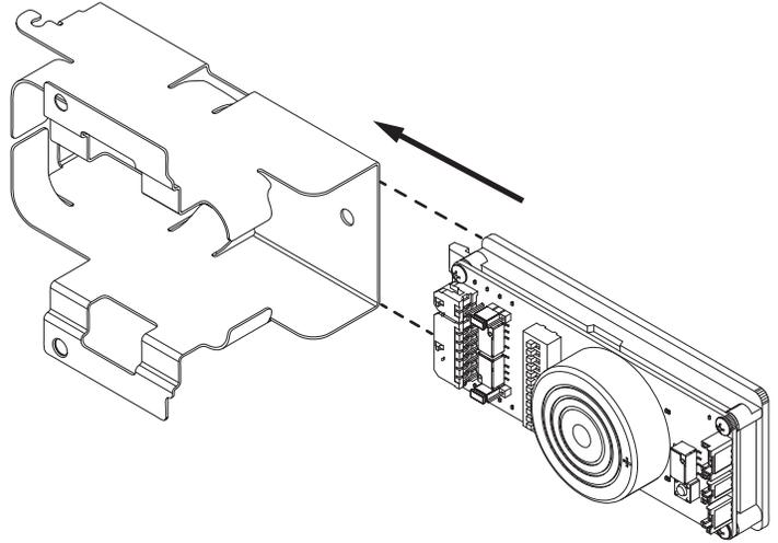
7l Route device wiring cable over mounting bracket and make connections on module per wiring diagrams in Section 4.
