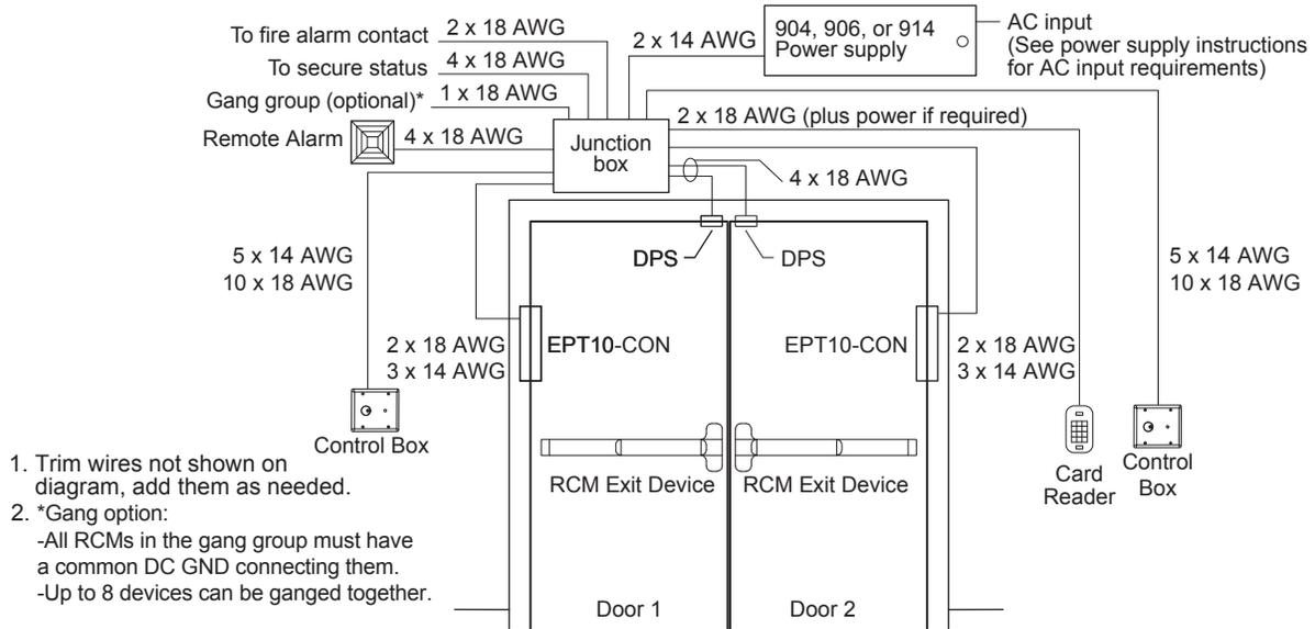
**Figure 3. Riser Diagram, Double Door**
