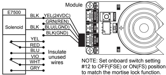
Access control to the RCM (not shown) inhibits the RCM and unlocks the E7500 mortise lock to allow entry. The E7500 can be either FS (Fail Safe) or FSE (Fail Secure). For access control wiring, see previous wiring diagrams.
