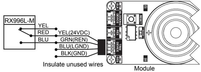
RX trim is not locked and allows entry at all times. The trim inhibits the RCM using the REN function during entry.
