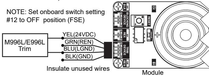
Access control to the RCM (not shown) inhibits the RCM and unlocks the outside FSE (Fail Secure) trim to allow entry. For access control wiring, see previous wiring diagrams.
