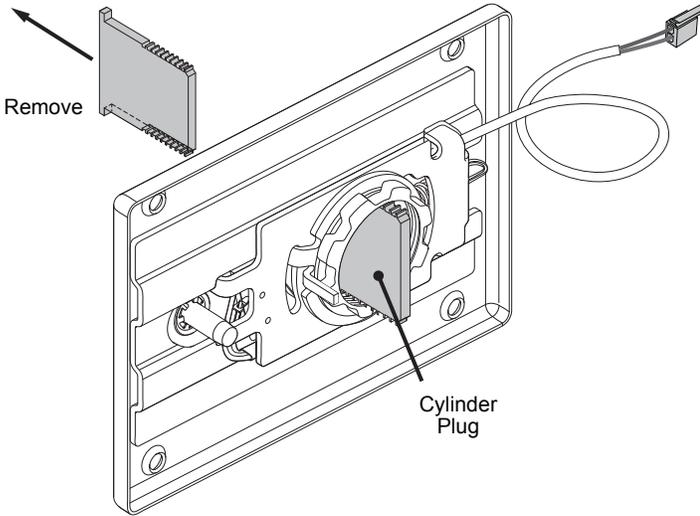
7n Use 1¼" mortise cylinder with compression ring K510-406 with straight cam and orient cam as shown. Schlage cylinder 20-001-114 recommended.
