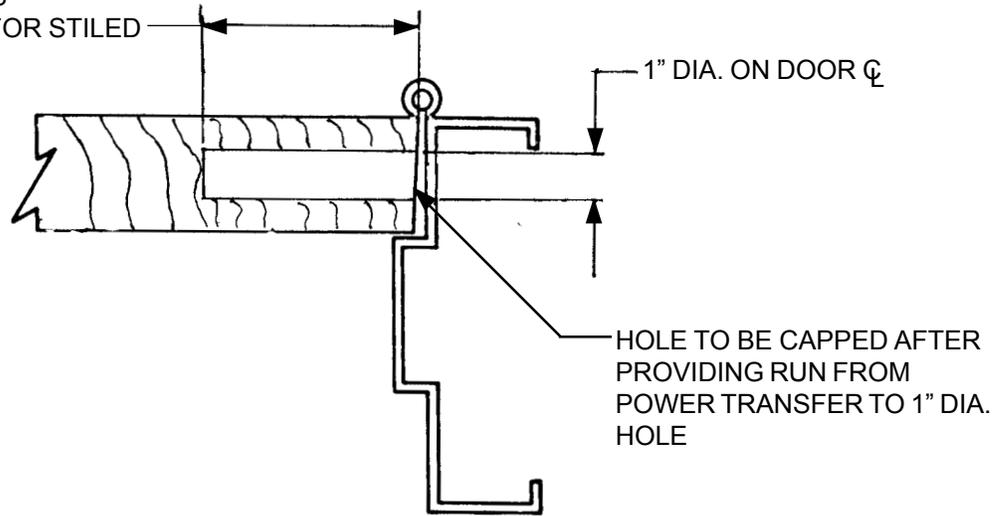
CLEAR CHANNEL ACCESS REQUIRED FOR WIRE CONNECTION
