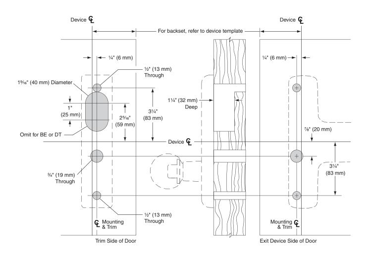
• For height from finished floor, refer to device template.
