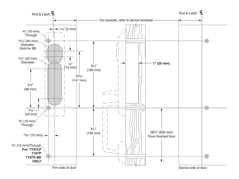
• For height from finished floor, refer to device template.
