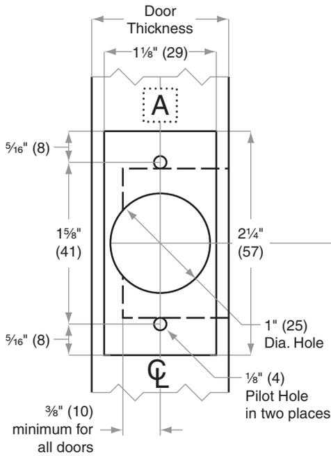
Dimensions shown in parentheses ( ) are in millimeters.
