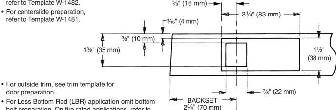
• For Less Bottom Rod (LBR) application omit bottom bolt preparation. On fire rated applications, refer to Template W-5494 for auxiliary fire latch preparation.
