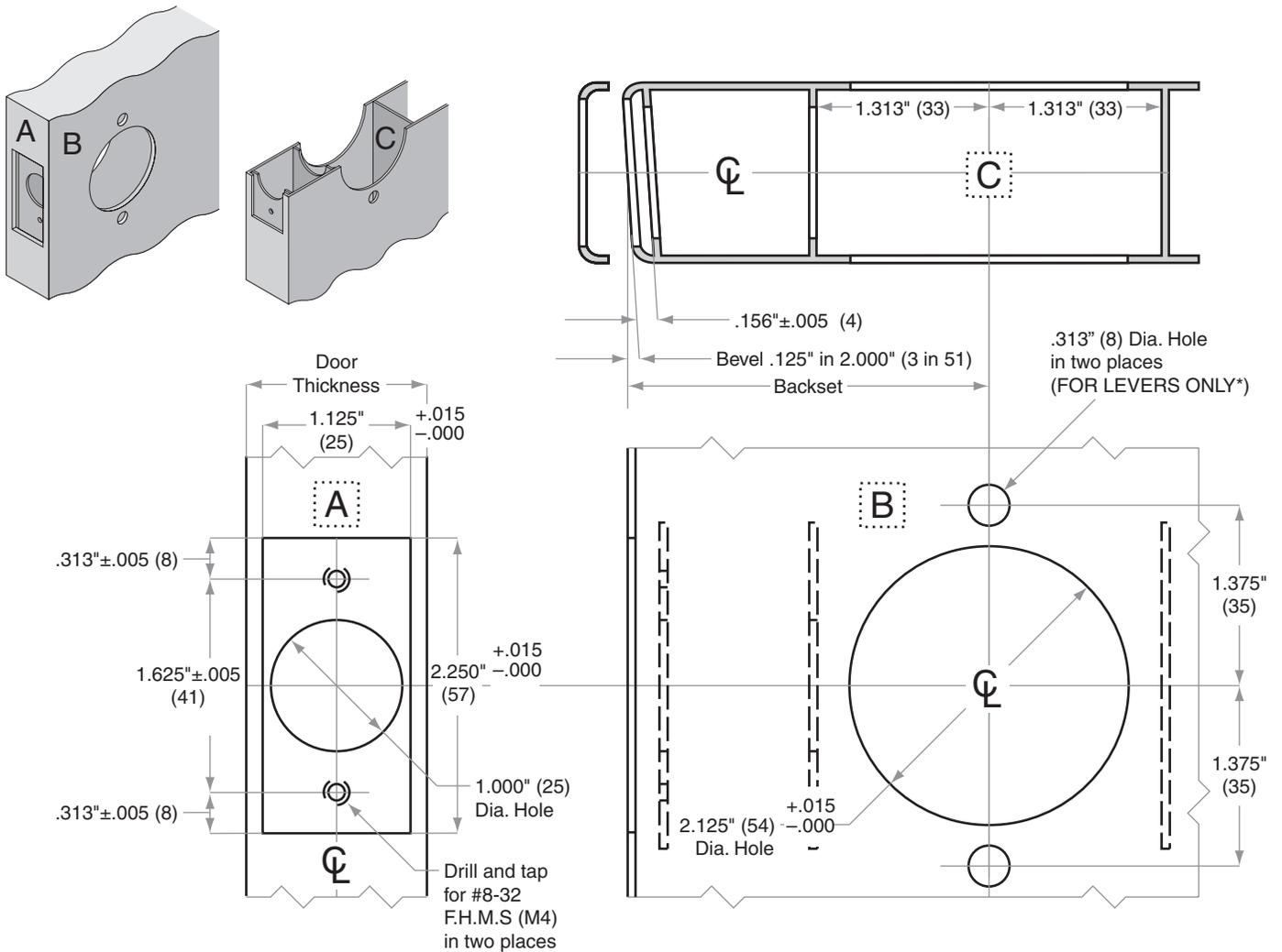
\*Mounting post holes are optional for levers only and cannot be used with knobs.
