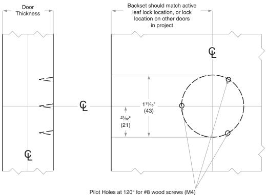
lot Holes at 120° for #8 wood screws (M Three holes, one side only
