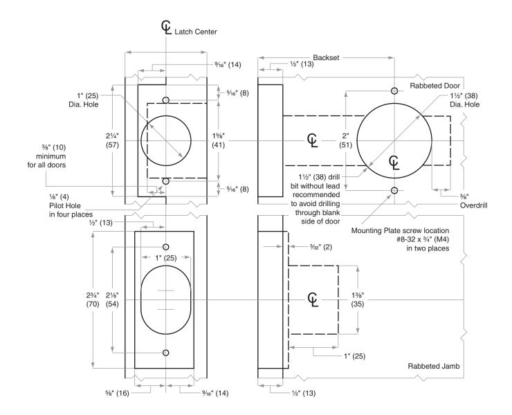
Dimensions shown in parentheses ( ) are in millimeters.
