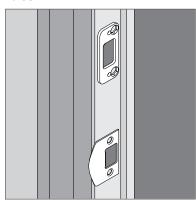
5b If correction is necessary, trace the faceplates and mark holes.
