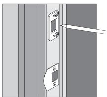
5c If necessary, use chisel, hammer and drill to correct door jamb preparation.
