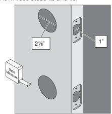
4b If necessary, enlarge holes in door face.
