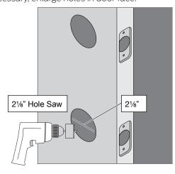
4c If necessary, enlarge holes in door edge.
