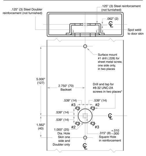
\*Drill two holes at locations #2 for outside RH/RHR or Drill two holes at locations #3 for outside LH/LHR
