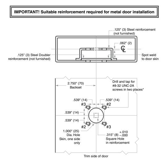
\* Drill and tap two holes at locations #2 for outside RH/RHR or inside LH/LHR doors or Drill and tap two holes at locations #3 for outside LH/LHR or inside RH/RHR doors
