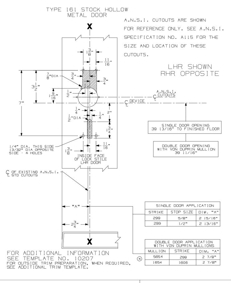
E98/E99 Series Rim Device w/ 990, 991, 992 Trim for Type "161" Stock Hollow Metal Applications
