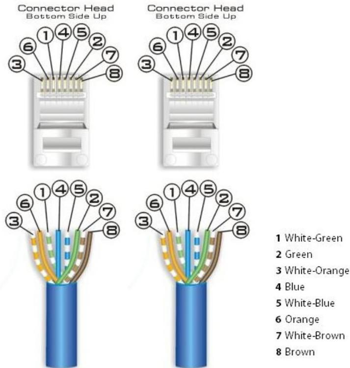
A standard Cat5e/6 cable is then run between the PoE source (Injector or switch) and the Pure IP Reader-Controller which will be located right next to the door. The Cat5e/6 cable can be up to 100 Meters (328 feet) long, including all patch cables and patch panels.
