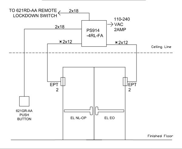
NOTES: 1) ALL LOW VOLTAGE WIRING TO BE STANDARD, MULTI-CONDUCTOR COLOR CODED WITHOUT SPLICES.
