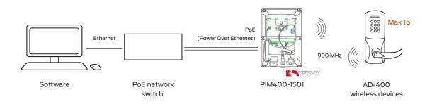
1 In order to have a UL Listed configuration a UL294 12VDC power supply must be used instead of PoE
