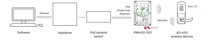
Wireless range up to 200' in typical building construction, up to 1000' line of sight
