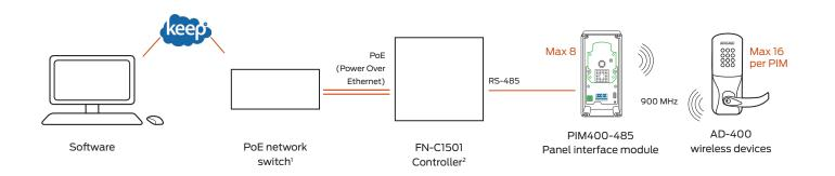
1 In order to have a UL Listed configuration a UL294 12VDC power supply must be used instead of PoE
