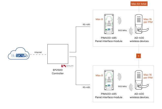
Wireless range up to 200' in typical building construction, up to 1000' line of sight
