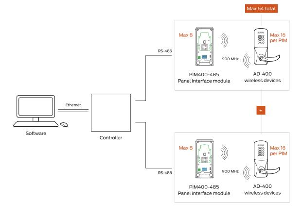
Wireless range up to 200' in typical building construction, up to 1000' line of sight
