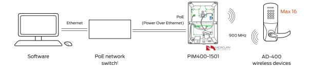
Wireless range up to 200' in typical building construction, up to 1000' line of sight
