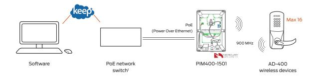
Wireless range up to 200' in typical building construction, up to 1000' line of sight
