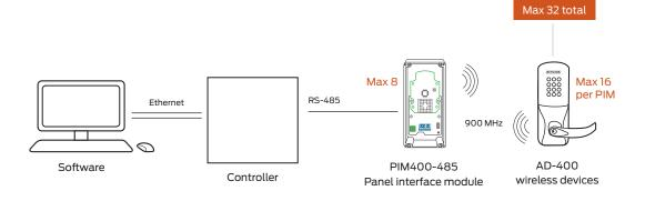
Wireless range up to 200' in typical building construction, up to 1000' line of sight
