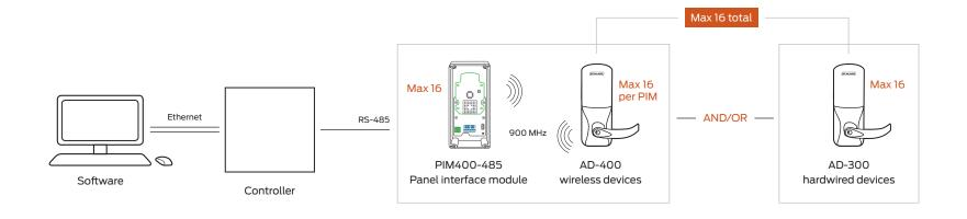
AD-400 wireless range up to 200' in typical building construction, up to 1000' line of sight.
