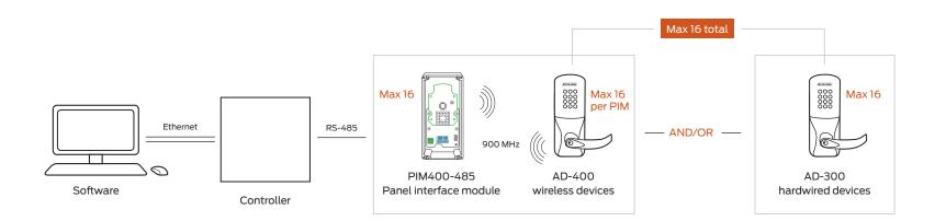
Wireless range up to 200' in typical building construction, up to 1000' line of sight
