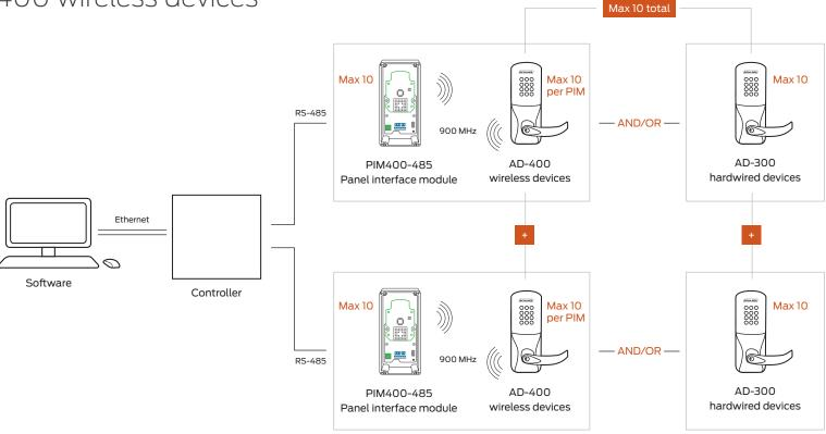
Wireless range up to 200' in typical building construction, up to 1000' line of sight
