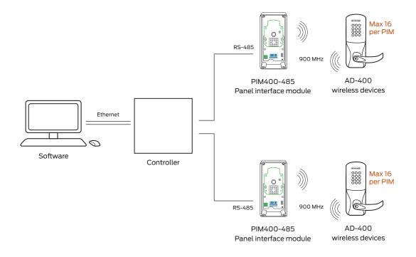
AD-400 wireless range up to 200' in typical building construction, up to 1000' line of sight.
