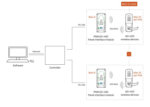
AD-400 wireless range up to 200' in typical building construction, up to 1000' line of sight.
