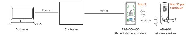
AD-400 wireless range up to 200' in typical building construction, up to 1000' line of sight.
