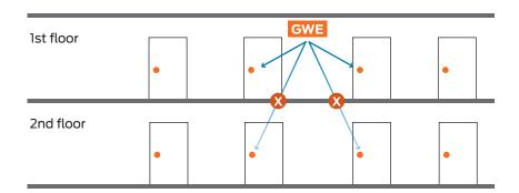
The wireless signal will not pass through metal walls or metal mesh in the walls (i.e. stucco).
