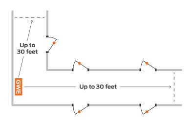
When planning an install for new construction where the building is not complete and fully operational, the planning should be based on the gateway being within 30 feet line of sight of the door. An additional 10% contingency should also be planned for with the number of gateways to support full coverage at the time of install
