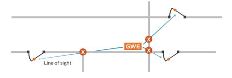
Do not mount the gateway and locks on different floors. The signal may be degraded and functionality could be severely limited.
