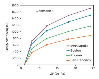
A recent study conducted by Purdue University examined the potential heating and cooling energy cost savings from using an effective closer. Looking at cities in varying climate zones, it found that by installing an effective closer on exterior doors, companies could save as much as \$1,695 annually per door in heating and cooling costs.
