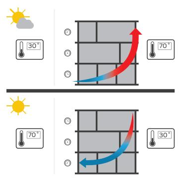
If the outdoor temperature is cooler than the indoor temperature, this can create an excessive amount of negative pressure within the lower levels of the building, and a correspondingly high level of positive pressure within the upper levels. The pressure difference pulls the cold outdoor air in at the lower levels and pushes the heated indoor air out at the upper floors. When it is warmer outdoors than indoors, the opposite happens.
