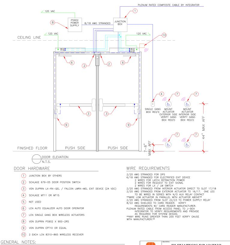
ALL LOW VOLTAGE WIRE TO RUN IN MINIMUM 3/4" CONDUIT OR INSIDE DRYWALL UNLESS NOTED OTHERWISE ALL LOW VOLTAGE WIRE TO BE STRANDED WIRE ALL GANG BOXES BY ELECTRICAL CONTRACTOR AS REQUIRED ALL LOW VOLTAGE WIRING TO BE LABELED CLEARLY AT BOTH END ALL MOUNTING HEIGHTS AS SHOWN COORDINATE MOUNTING LOCATIONS WITH ELECTRICAL/ARCHITECTURAL PLANS ANY DEVIATION FROM HARDWARE SPECIFIED IN SECTION 08710 WILL NEGATE ALL REQUIREMENTS SHOWN HEREIN AND REQUIRE NEW DRAWINGS BY OTHERS TO MATCH SUBSTITUTED HARDWARE
