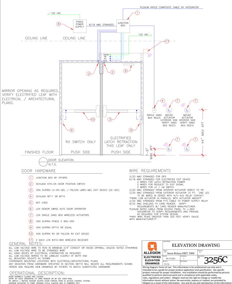
DOR NORMALLY CLOSED AND LOCKED. ENTRY BY VALID CREDENTIAL AT CARD READER OR BY KEY OVER-RIDE. RX SWITCH / MOTION SENSOR SHUNTS DOOR FORCED OPEN IN ACCESS CONTROL SYSTEM. INTERIOR ACTUATOR TO START OPENING CYCLE (UNLESS ADD IS POWERED OFF) EXTERIOR ACTUATOR WIRED IN SERIES THROUGH LX SWITCH IN EXIT DEVICE SUCH THAT ON VALID CARD OR TIME ZONE CONTROL ACTUATOR CON BE PRESSED TO START OPENING CYCLE KEY OVER-RIDE WILL CAUSE DOOR FORCED EVENT IN ACCESS CONTROL SYSTEM. FREE EGRESS AT ALL TIMES.
