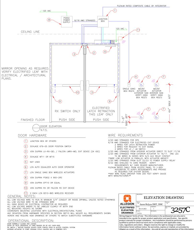
DOOR NORMALLY CLOSED AND LOCKED. ENTRY BY VALID CREDENTIAL AT CARD READER OR BY KEY OVER-RIDE. RX SWITCH / MOTION SENSOR SHUNTS DOOR FORCED OPEN IN ACCESS CONTROL SYSTEM. INTERIOR ACTUATOR TO START OPENING CYCLE (UNLESS ADD IS POWERED OFF) EXTERIOR ACTUATOR WIRED IN SERIES THROUGH LX SWITCH IN EXIT DEVICE SUCH THAT ON VALID CARD OR TIME ZONE CONTROL ACTUATOR CAN BE PRESSED TO START OPENING CYCLE KEY OVER-RIDE WILL CAUSE DOOR FORCED EVENT IN ACCESS CONTROL SYSTEM. FREE EGRESS AT ALL TIMES.
