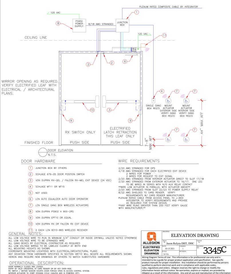
DOOR NORMALLY CLOSED AND LOCKED. ENTRY BY VALID CREDENTIAL AT CARD READER OR BY KEY OVER-RIDE. RX SWITCH / MOTION SENSOR SHUNTS DOOR FORCED OPEN IN ACCESS CONTROL SYSTEM. INTERIOR ACTUATOR WIRED IN SENEST STRUCH ACCESS CONTROL SYSTEM AUX RELAY SUCH THAT ON VALID CARD OR TIME ZONE CONTROL ACTUATOR WIRED IN SENESS THROUGH ACCESS CONTROL SYSTEM AUX RELAY SUCH THAT ON VALID CARD OR TIME ZONE KEY OVER-RIDE WILL CAUSE DOOR FORCED EVENT IN ACCESS CONTROL SYSTEM. FREE EGRESS AT ALL TIMES.
