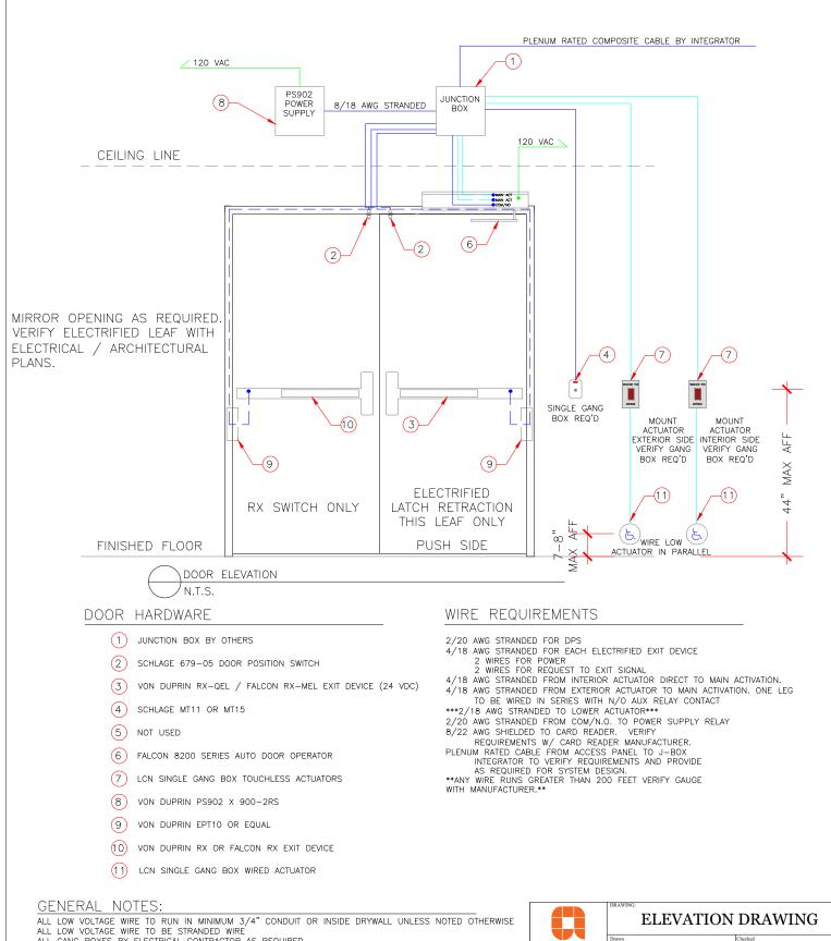
ALL GANG BOXES BY ELECTRICAL CONTRACTOR AS REQUIRED ALL LOW VOLTAGE WIRING TO BE LABELED CLEARLY AT BOTH END
