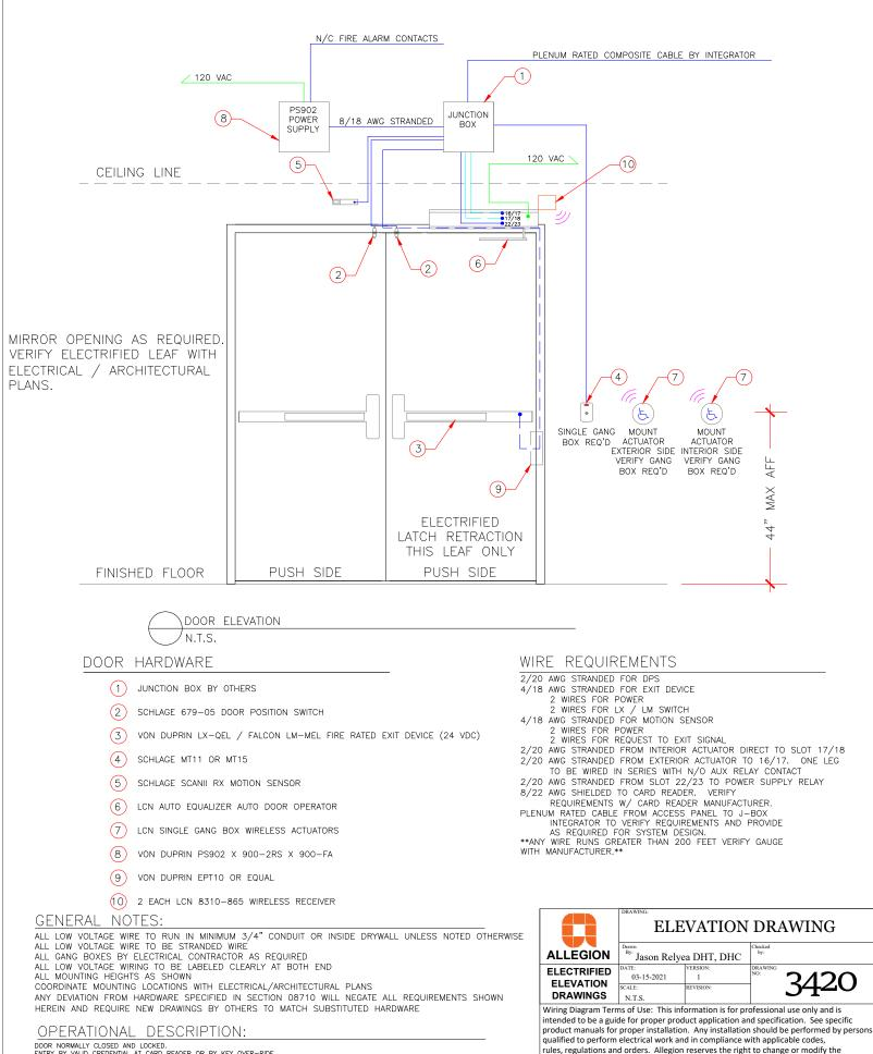
DOR NORMALLY CLOSED AND LOCKED. ENTRY BY VALID CREDENTIAL AT CARD READER OR BY KEY OVER-RIDE. RX MOTION SENSOR SHURTS DOOR FORCED OPEN IN ACCESS CONTROL. SYSTEM. INTERIOR ACTUATOR TO START OPENING CYCLE (UNLESS ADD IS POWERED OFF) EXTERIOR ACTUATOR WIRED IN SERIES THROUGH LX SWITCH IN EXIT DEVICE SUCH THAT ON VALID CARD OR TIME ZONE CONTROL ACTUATOR CAN BE PRESSED TO START OPENING CYCLE KEY OVER-RIDE WILL CAUSE DOOR FORCED EVENT IN ACCESS CONTROL SYSTEM. FREE EGRESS AT ALL TIMES.
