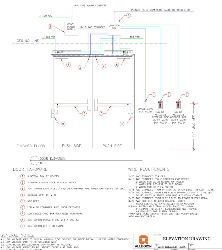
ALL GANG BOXES BY ELECTRICAL CONTRACTOR AS REQUIRED ALL LOW VOLTAGE WIRING TO BE LABELED CLEARLY AT BOTH END ALL MOUNTING HEIGHTS AS SHOWN
