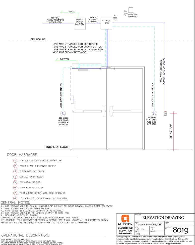
DOOR NORMALLY CLOSED AND LOCKED. ENTRY BY VALID CREDENTIAL AT CARD READER OR BY KEY OVER-RIDE. PIR MOTION SENSOR SHUNTS DOOR FORCED OPEN IN ACCESS CONTROL SYSTEM. INTERIOR ACTUATOR TO START OPENING CYCLE (UNLESS ADD IS POWERED OFF) EXTERIOR ACTUATOR WIRED IN SERIES THROUGH ACCESS CONTROL SYSTEM AUX RELAY SUCH THAT ON VALID CARD OR TIME ZONE CONTROL ACTUATOR CAN BE PRESSED TO START OPENING CYCLE. KEY OVER-RIDE WILL CAUSE DOOR FORCED EVENT IN ACCESS CONTROL SYSTEM. FREE EGRESS AT ALL TIMES.
