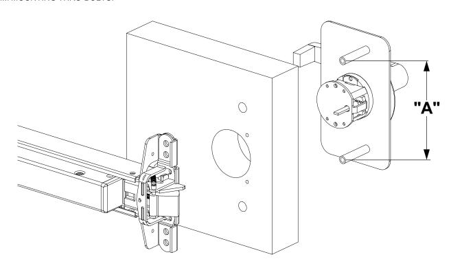
3) IF"A" ABOVE IS 3-1/2", PREPARE THE HOLES MARKED **"B" (INSTEAD OF "A")** IN THE INSTALLATION INSTRUCTIONS. IF "A" ABOVE IS 4-1/2", PREPARE THE HOLES PER THE INSTALLATION INSTRUCTIONS.
